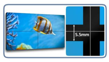
Seamless Video Wall - With a total bezel size as narrow as 5.5mm these displays are ideal as part of a virtually seamless LCD Video Wall – keeping all of the focus on your content.
